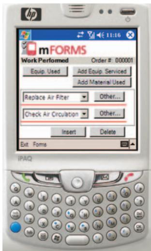
**Drop-down forms on the technician’s handheld computer can make the input of job site information a simple “multiple-choice”.**
