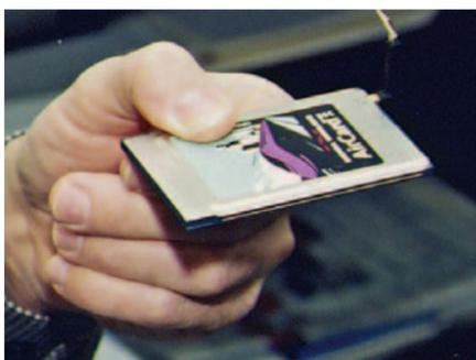
**An air card is used to connect a laptop to a wireless network.**
